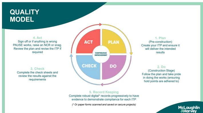
The subcontractor shall provide Quality Plans, Programmes, Inspection & Test Plans (ITPs), Check Sheets and any associated quality records and check sheets in relations to all elements of their works, or works subcontracted by them.
